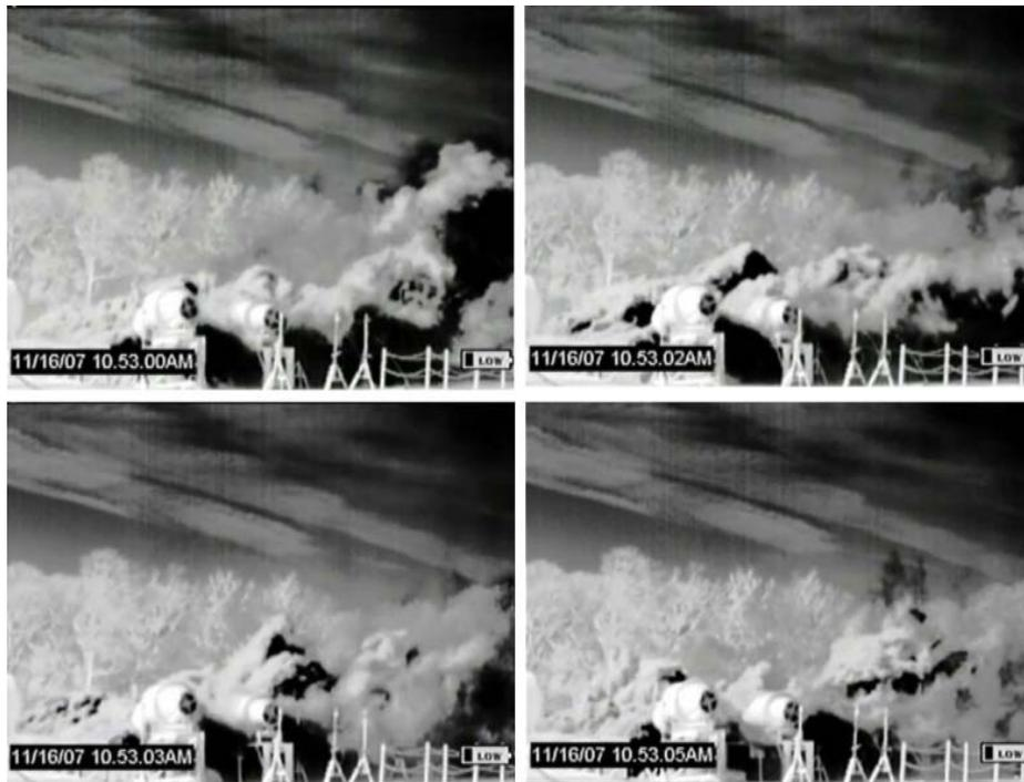
**Figure 1.** LNG cloud from LNG spill on concrete visualized by infrared camera.
