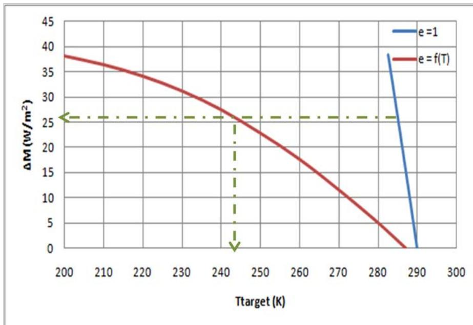
**Figure 3.** Actual target temperature vs. apparent target temperature from the thermogram
