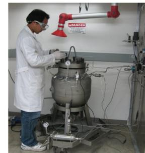
36-L Dust Explosion Apparatus
